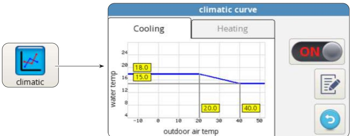
To optimize energy saving, two climatic curves are available, one for heating and one for cooling. These curves allow to adjust water temperature to external air temperature and, therefore, thermal load.
