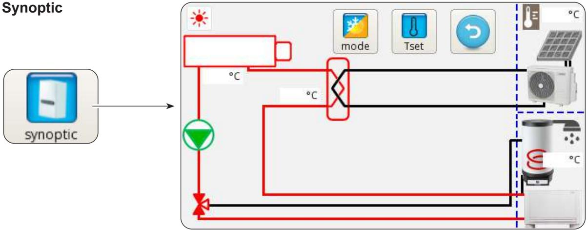
The synoptic shows the system diagram and operating status in real time.
