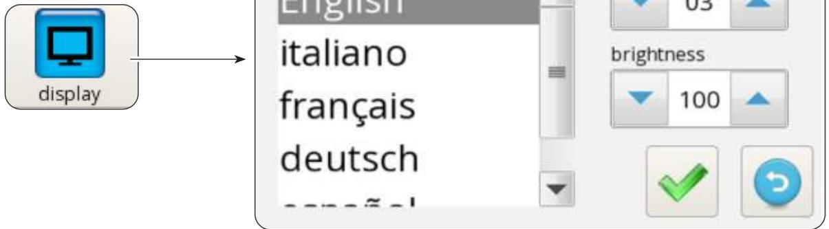
This screen allows to select the language, to set the start delay time of the screensaver function and to set the screen brightness.
