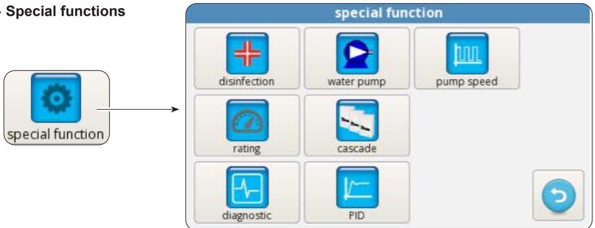
The special functions screen includes a series of functions and controls for configuration and monitoring of the heat pump.
